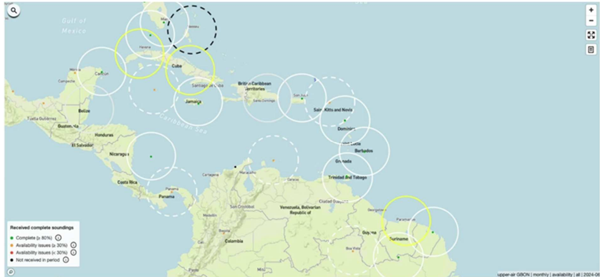
Figure 4 GBON 500km Standard Upper Air circles applied to stations across the Caribbean on WQMS (as opposed to larger 1000km circles for the Eastern Caribbean states if considered under SIDS criteria)
