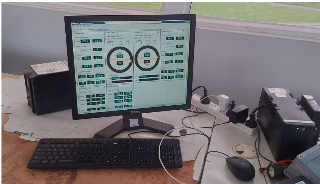
Figure 9. Faleolo observations office display of the two JICA AWSs located at each end of the runway. A second display is available in the Air Traffic Control Tower.
