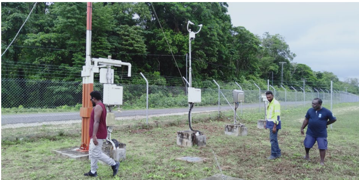
Figure 4 Automatic weather observing system (AWOS) at Munda Airport with CAASI personnel
